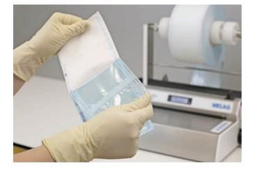
Please make sure to carry out the peel test on a **daily** basis, preferably before starting work: The tested seal seam must be even and complete.
