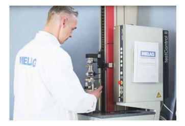
In order to validate packaging processes and to evaluate the performance of sealing devices, hygiene experts strongly recommend the seal seam stability test as an **annual** routine check.
