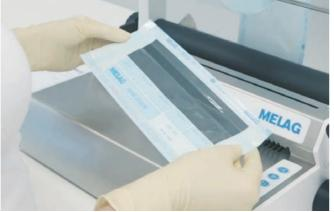
The **weekly** seal check verifies the quality of the seal seam in accordance with DIN EN ISO 11607-2.
