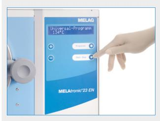
The MELA*tronic*®23 EN is equipped with four sterilization programs. The Universal-Program "S" and Prion-Program "S" (both 134 °C) are intended for the sterilization of small quantities of wrapped massive instruments. The Quick-Program "N"(134 °C) can be used to sterilize unwrapped instruments; the Gentle-Program "N" uses a low temperature of 121 °C to sterilize temperature-labile, massive instruments (unwrapped).
