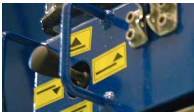
Joystick in each corner controls lift and tilt - no need for remote control
